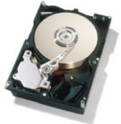
IBM Ultrastar 9LZX 3.5-inch low-profile Ultra2 SCSI (LVD) 9.1 GB 10,020 RPM disk drive
